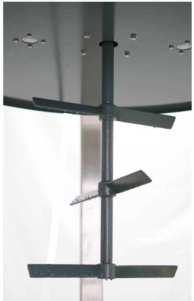
Figure 2 : Teflon coated paddle impellers for corrosive application.
