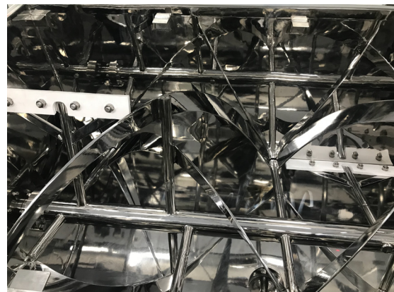
Figure 2 : Double helical ribbon design with Teflon scraper
