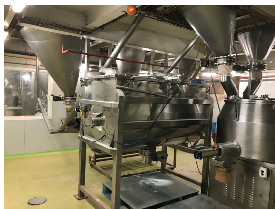
Figure 3 : Ribbon Blender with vacuum feeders on top.
