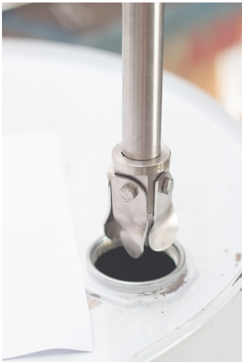
Figure 3: "Collapsible" folding impellers for entry to all standard drum containers.
